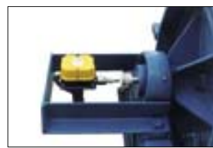
Ontcoder + spindelstop Encoder + spindle limit switch
